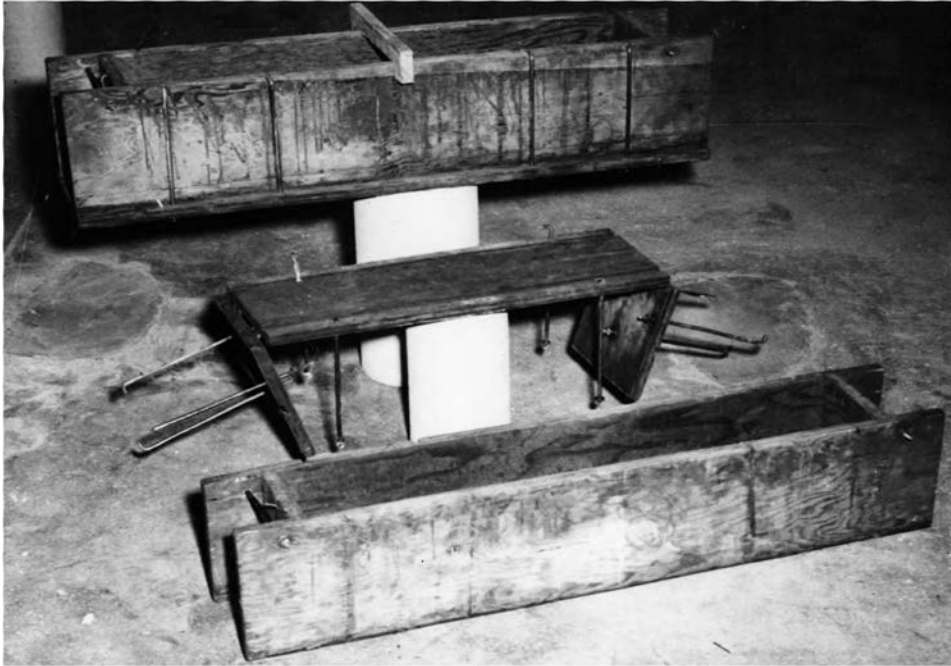
FIGURE 3 - BEAM FORM - LAID OUT AND ASSEMBLED
