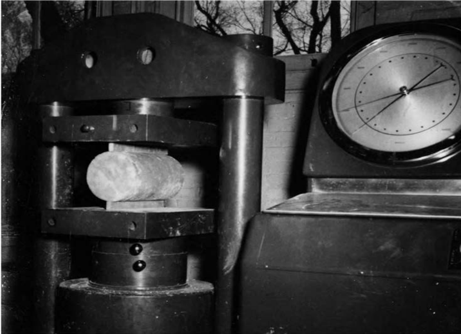
FIGURE 6 - CYLINDER IN PLACE FOR INDIRECT TENSILE TEST
