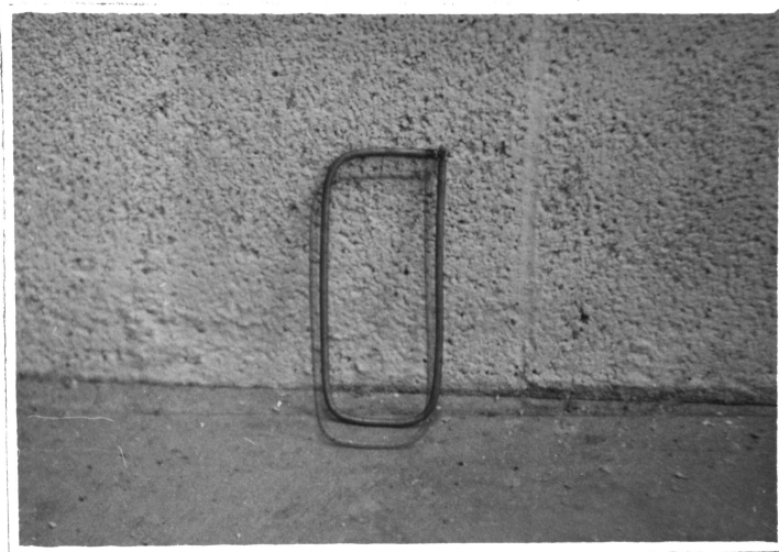
FIG. 14 CLOSED LOOP STIRRUP DETAIL
