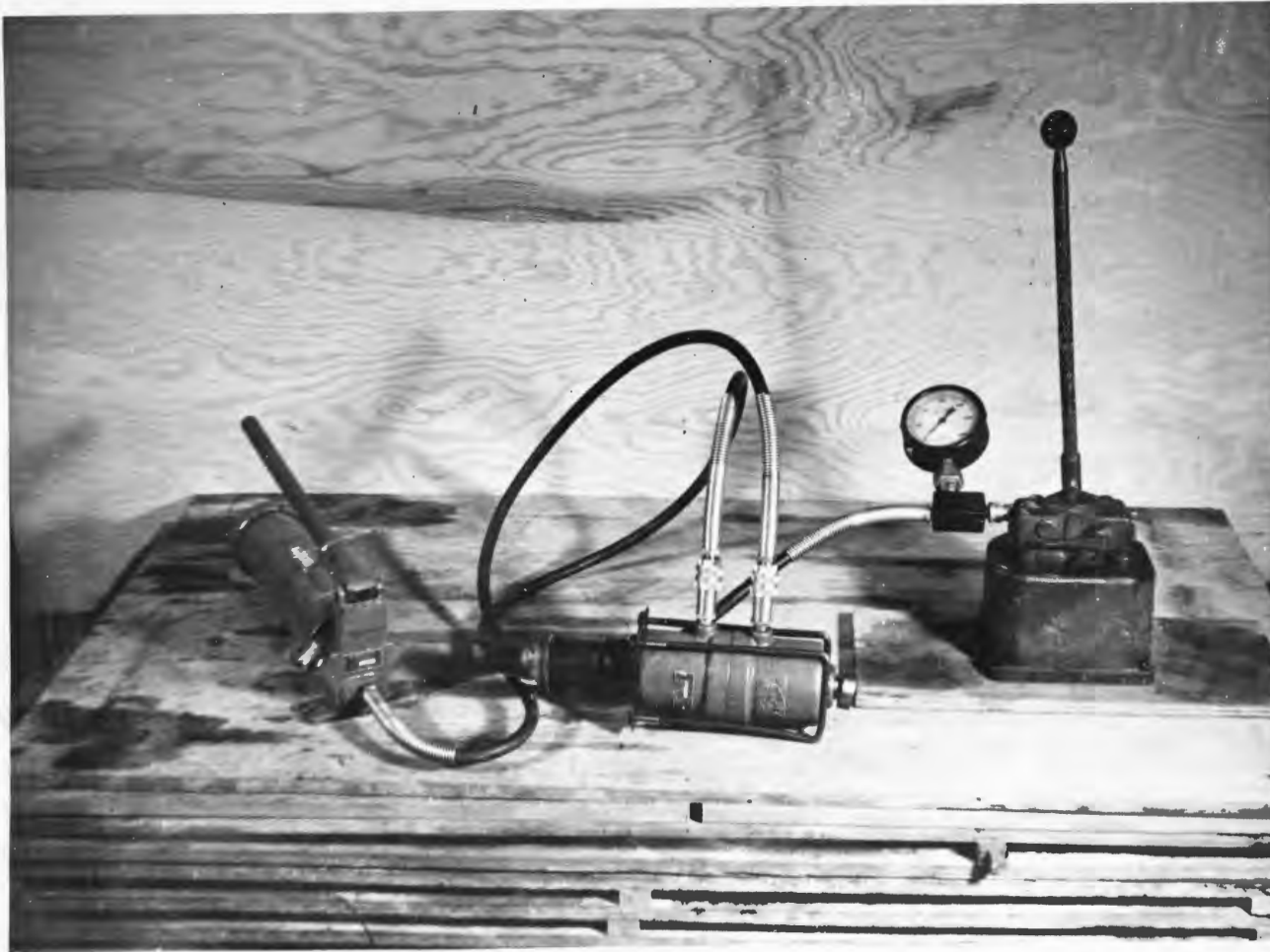
Fig. 25 Jacking unit. Left to right: Simplex pump to activate pushing ram, hose connections, prestressing unit, hydraulic pump to activate pulling ram.
