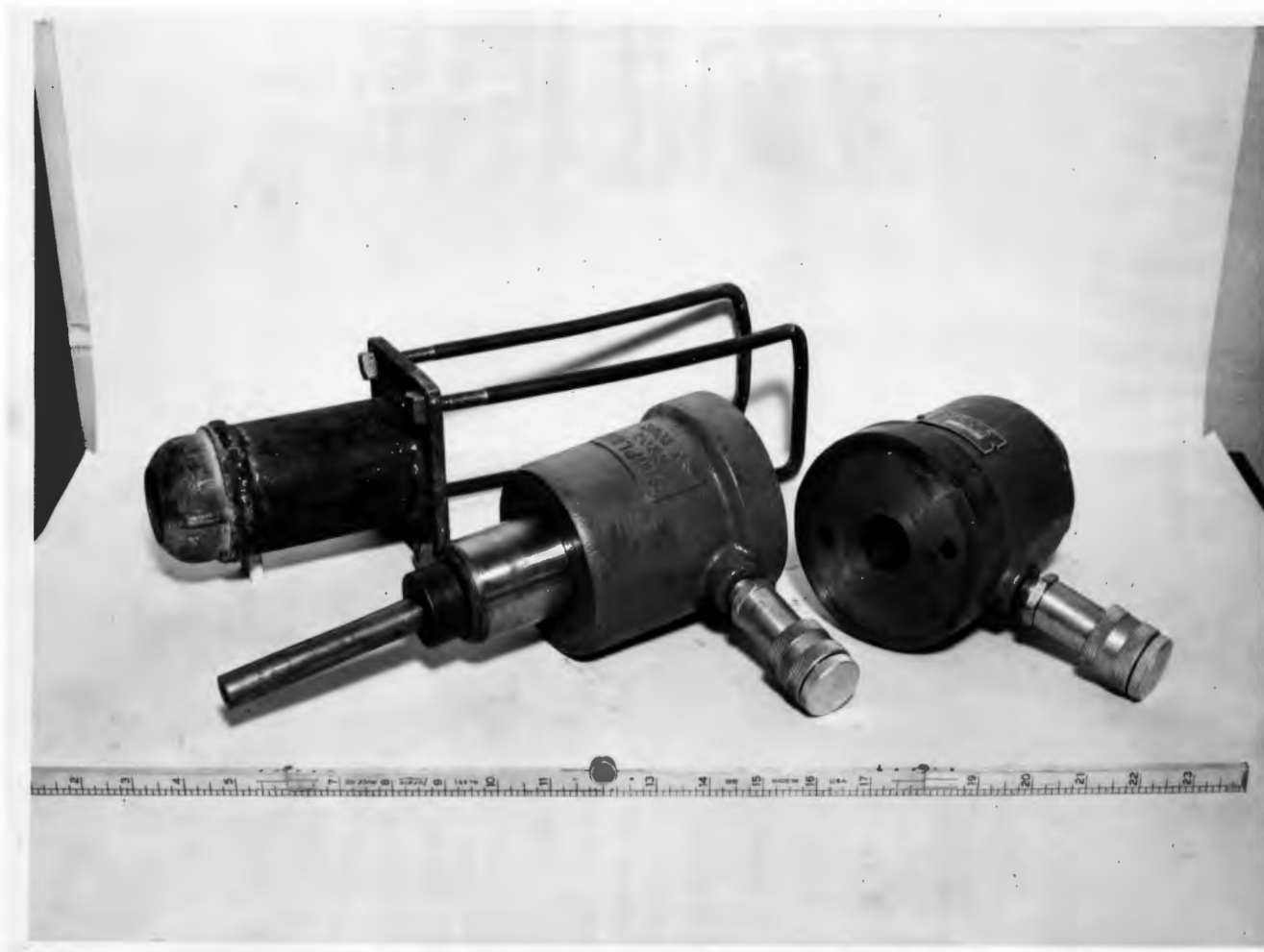
Fig. 23 Component parts of prestressing unit. Left to right: stand-off unit, pushing ram with follower, pulling ram.
