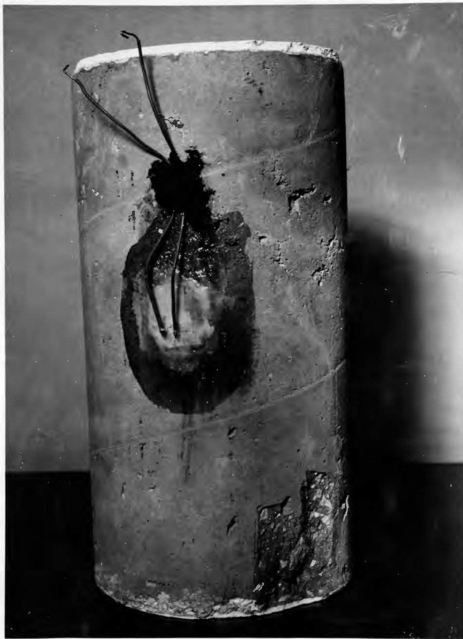
Fig. 18 Cylinder No. 2 after loading to limit of testing machine--7070psi. Small flaked-off area near bottom was only indication of failure. Note SR-4 Strain Gage.
