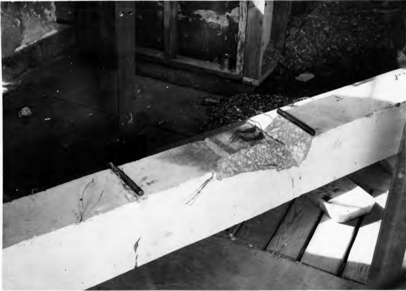
Fig. 38 Beam after removal of loading assembly, showing location and extent of crushing zone.
