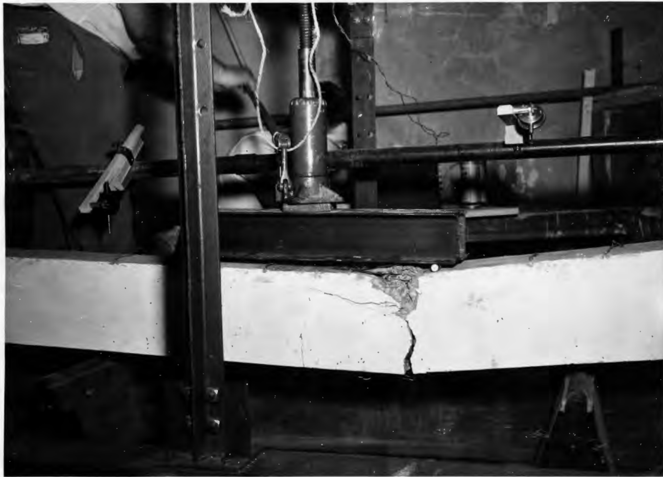
Fig. 36 Beam under load after four of five wires had failed. Deflection approximately 5-in. Beam returned nearly to normal after removal of this load.
