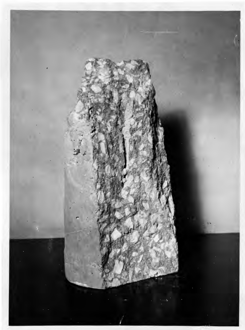
Fig. 20 Cylinder No. 5 Breaking strength 190,660 lbs.--6730 psi.
