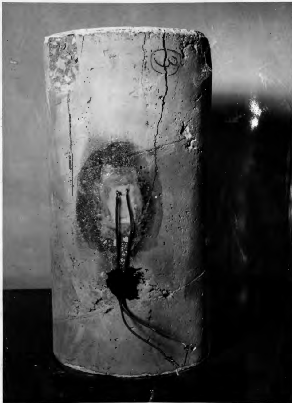
Fig. 19 Cylinder No. 4 after failure: stress-6855 psi. Note SR-4 Strain Gage on side.
