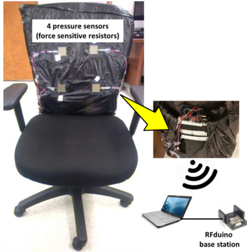
Figure 3.5. Overall Care-Chair system design
