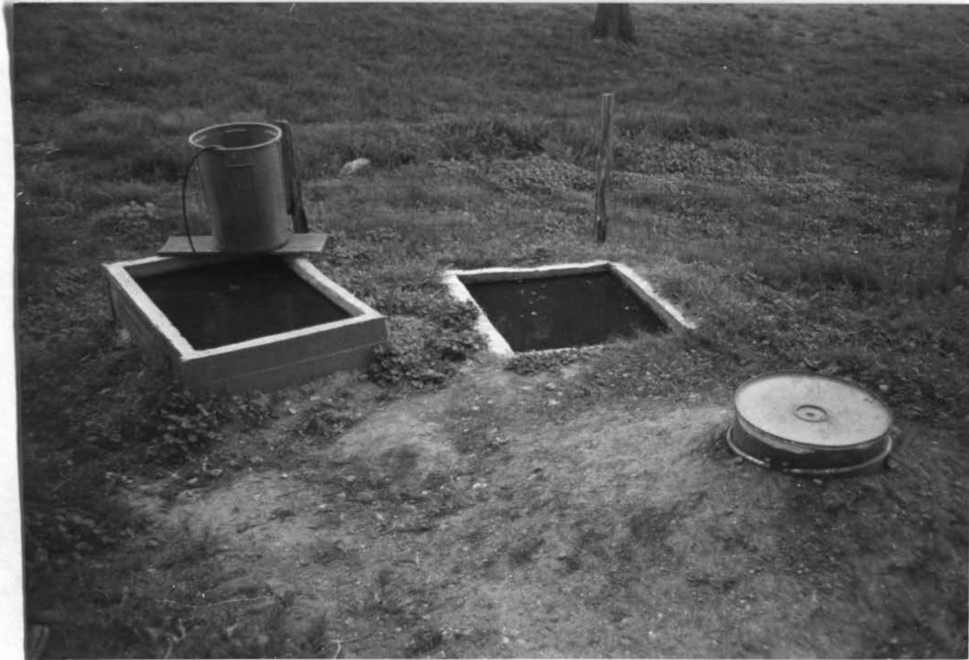
From left to right: dual (with feeding barrel), aerobic, and anaerobic lagoons
