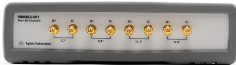
Figure 1.1. Traditional Channel Emulator Agilent M8048A [3]
