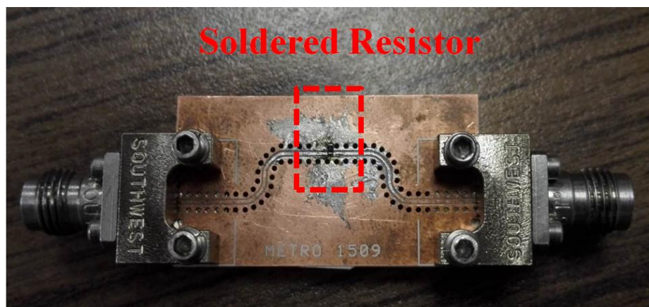
Figure 4.9. DUT to Investigate Solder Parasitic Effect
