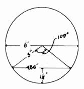
Area = area sector - area triangle.  $= \frac{109}{360} \times \frac{3.1416}{4} \times \frac{25}{2} - \frac{4.86}{2} \times \frac{1.75}{2}$ = .0304 sq. ft. Wetted perimeter =  $\frac{109}{360} \times 2 \times 3.1416 \times .25$ = .475 ft. R = .0304 = .0619 VR = .249V = cVRS = 85 x .249 x .1 = 2.12 ft/sec $Q = 60 \text{ AV} = 60 \text{ x} \cdot 0304 \text{ x} 2 \cdot 12 = 3.37 \text{ cu ft/min}$ . Estimated discharges for these lines are 3.96 and 3.94 cu.ft/min respect-
