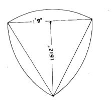
Area equi.  $\triangle = \frac{1.512}{2} \times 1.3/4 = 1.323$  eq.ft. " sector =  $\frac{3.1416}{6 \times 4} \times (3.5)^2$  = 1.604 " " " segment = 1.604 - 1.323 = .28 " " Total Area =  $1.323 + 2 \times .28 = 1.883$  " " Perimeter of sector =  $2 \times 3.1416 \times 1.75$ 6 = 1.83 feet.
