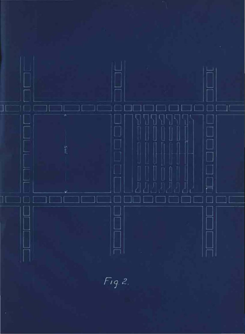
In the panel system no rooms are turned from the cross entries, but stub entries are driven every 500 feet at right angles to the cross entries, thus dividing the mine into blocks or panels which are 500 feet square. Eight rooms are usually turned off the stub entries, leaving sufficient barrier pillars for the protection of the cross entries.
