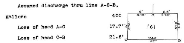
Equivalent diameter of pipe, 1980 ft. long, which will give a loss of head of 39.3 feet when discharging 400 gallons, is 5.8 inches.
