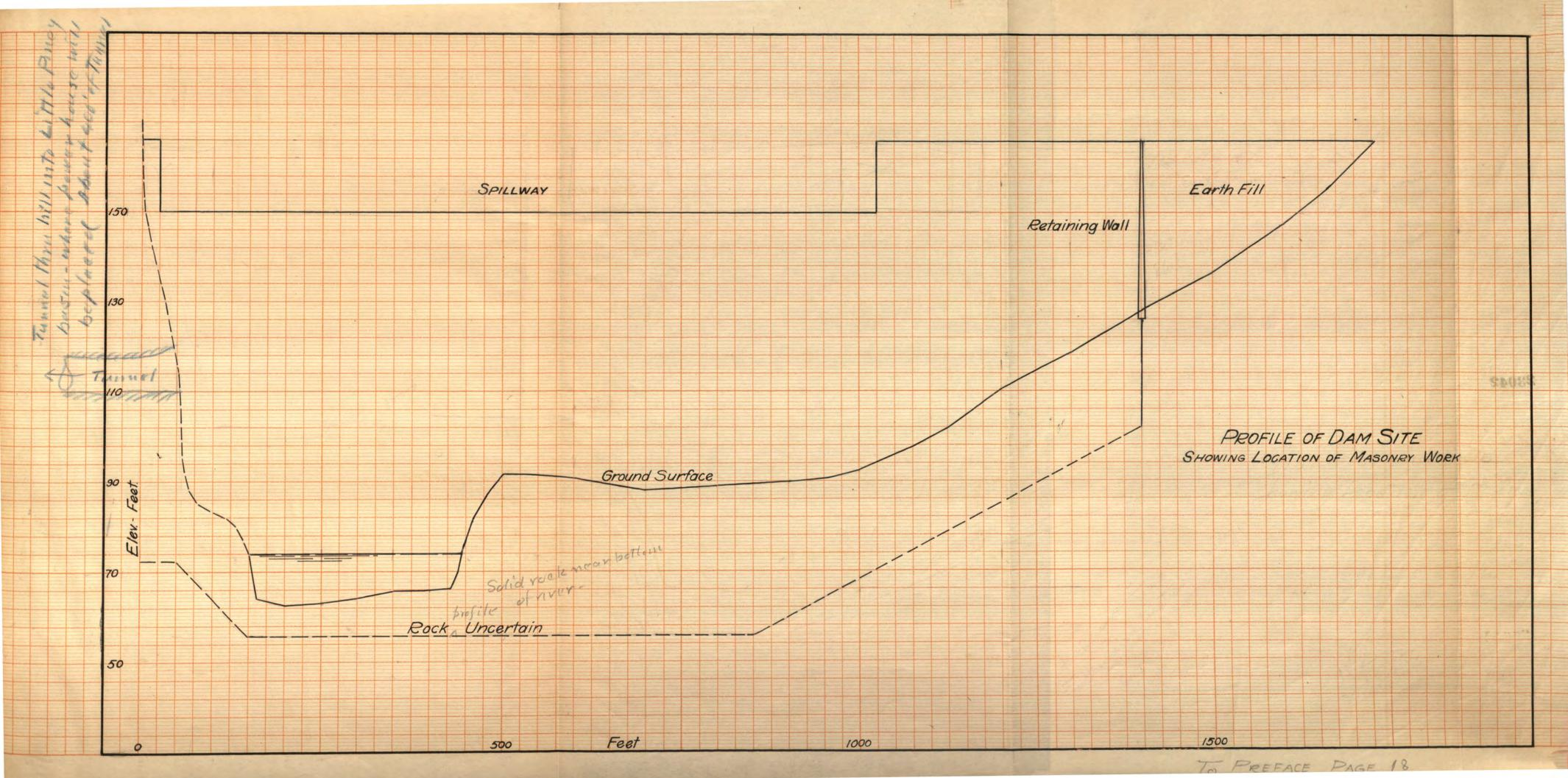
The subject of a foundation cannot be dismissed so easily. It is regretable to say that during the time that soundings were being taken, the river was at such a stage that it was impossible to reach solid rock by any means available. In going on with this work the assumption was made that rock could be found at a depth of ten feet below the river bed. This assumption is reasonable, because a few hundred feet below the site rock bottom is found only a few feet below the river bed.
