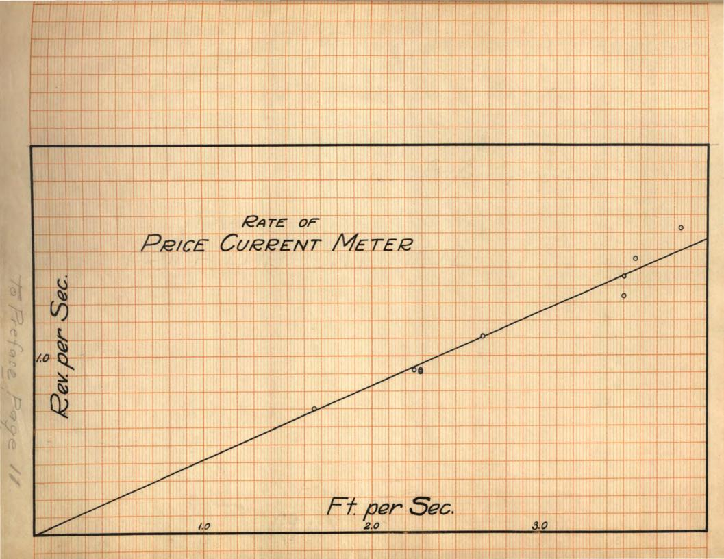
time. This work was done independently of the work of getting the velocity of the boat. From these results the velocity in feet per second was plotted as abscissae, and revolutions per second as ordinates, which gave a straight line curve. With this curve it is possible to compute the velocity in feet per second from the revolutions of the water meter.
