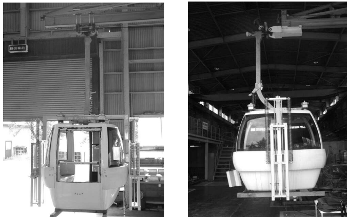
Fig. 12. Pictures of gondola with absorbers
