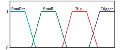
Fig. 5. Membership function proposed for the fundamental frequency amplitude and the spectral energy.
