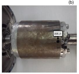
(c) Fig. 4. (a) Misalignment. (b) Unbalance. (c) Broker rotor bar.
