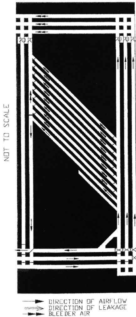
Figure 4. Generalized bleeder system for proposed thin-seam panel.
