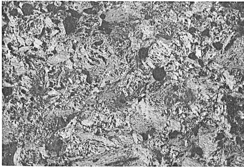
FIGURE 6. REPRESENTATIVE MICROSTRUCTURE OF CONVENTIONALLY FABRICATED REACTOR-GRADE GRAPHITE
