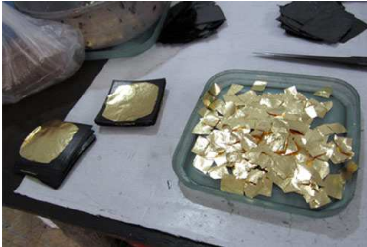
Fig. 1. The thin gold leaves fabricated by the traditional laminating technology.
