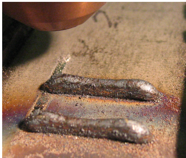
Figure 2: Semi-Automatic Deposition of a 20 Layer Thin Wall Structure
