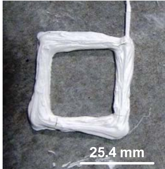
Figure 24: Square part fabricated with extrusion force controller and a constant reference force of F_r = 311\text{ N} .
