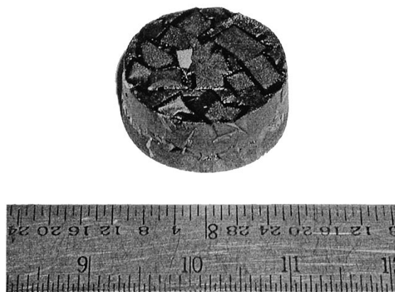
Fig. 2. Melt textured Y123 processed with 2.0 mol% neodymium oxide.
