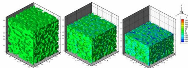
**Figure 3.** 3D views of foam RVE in compression from MPM simulation.
