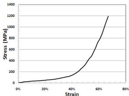
**Figure 4.** Compression of stress strain curve obtained from numerical simulation using MPM. The stress strain relation at small strains is shown in Figure 2.
