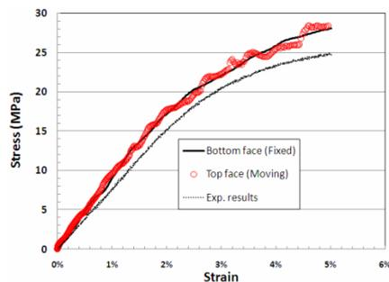
**Figure 2.** Compressive stress-strain curves from the MPM simulation showing the dynamic equilibrium.
