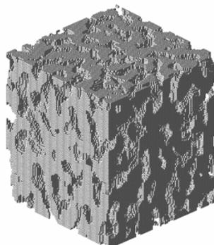
**Figure 1.** 3D discretized MPM model for a crosslinked template silica-aerogel (X-MP4-T045) by converting the grayscale n-CT information into material points.
