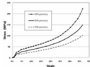
**Figure 5.** Compressive stress-strain curve for model with different porosity obtained from numerical simulation using MPM. The curves follow a cubic power relation with density.
