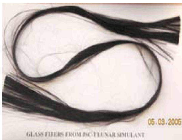
FIGURE 9. Glass Fibers Prepared from JSC-1 Lunar Simulant. Typical Diameters of Individual Fibers Vary Between 15 to 30 \mu\text{m} .
