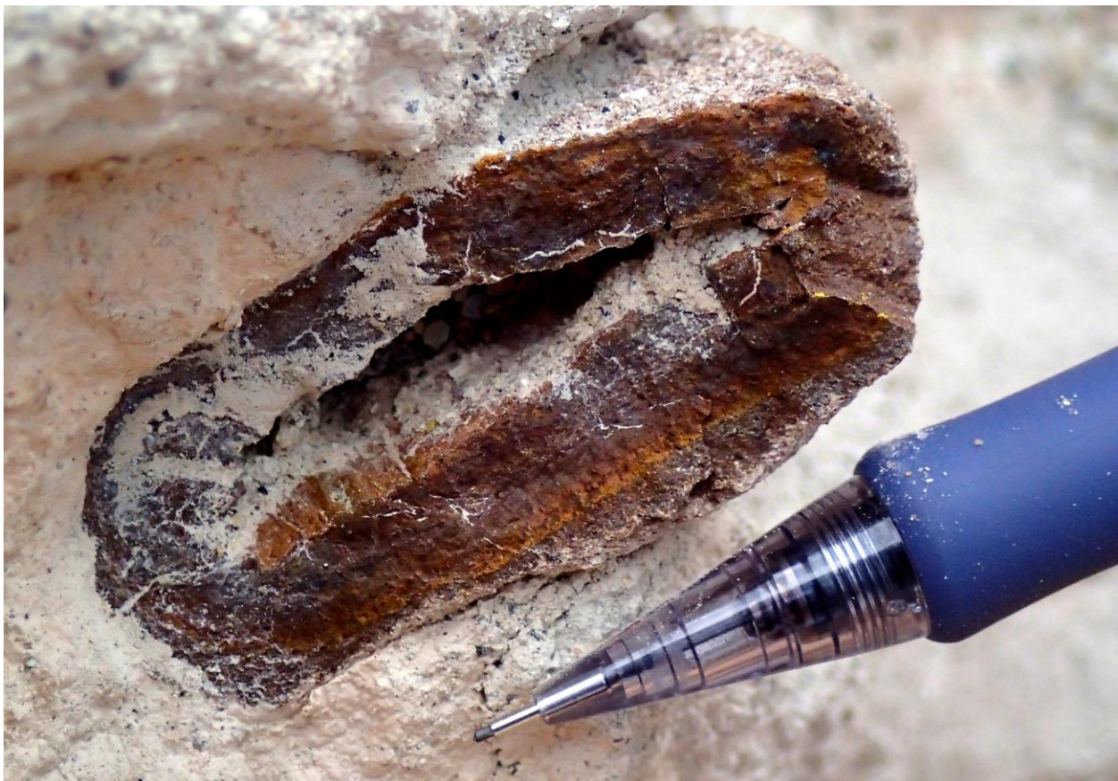
Figure 8. The entrained wood specimens in less competent layers exhibit distinct evidence of plastic deformation through modification of transverse surfaces from round to elliptical forms. Red-brown coloration is typically associated with fragmentation, dissolution of organic materials, and lack of structural definition. This sample, as was common in others, also lacked a central mass.
