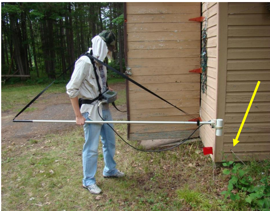
Figure 6. Checking to verify electricity turned off. Arrow points to electric line to garage. Photo by K. J. Neuhauser.
