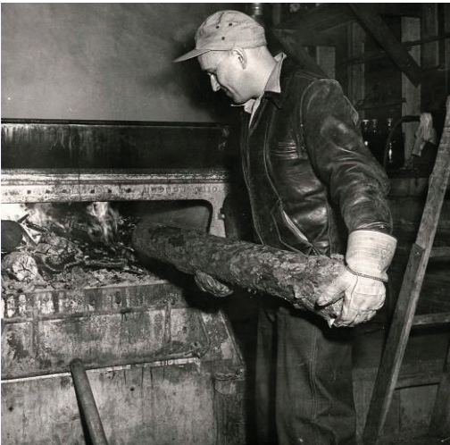
Figure 3. Brother John Anderl putting a log in the firebox of the evaporator in the original sugar house in 1955. Note that the stove is elevated about 16 inches. Image by permission of St. John's Abbey Archives.
