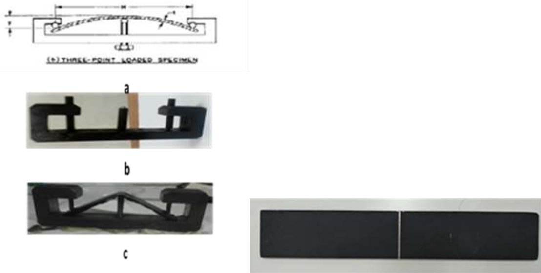
d. Samples of 5L-X6 API test specimens. Figure 1. Holder shape and mounting of test specimen.
