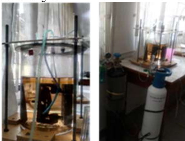
Figure 2. Chamber corrosion test.
