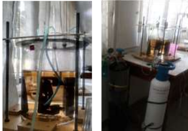
Figure 3. Chamber corrosion test. (a container tube white is H 2 S gas and container tube black is CO 2 gas) at room temperature.
