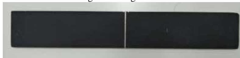
Figure 2. The plate samples test corrosion API 5L-X65 were initially cracked.
