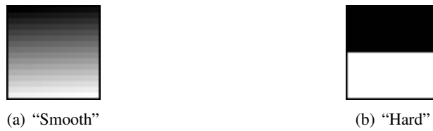
Figure 7: Test images for sparsity index boundaries evaluation. (a) sparsity index is equal to 0 and (b) is equal to 2.
