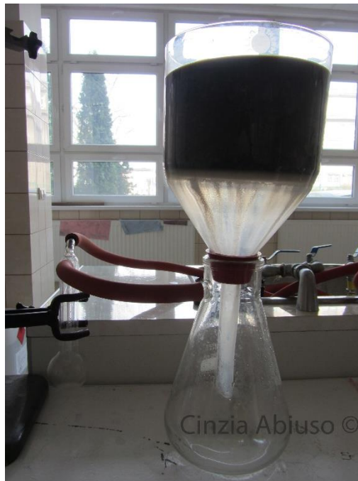
Figure 9.1 - Glass funnel with diatomaceous earth and charcoal (1:1 w/w)
