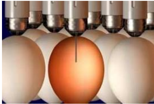
Figure 5.1 - Schematic representation of in ovo injection
