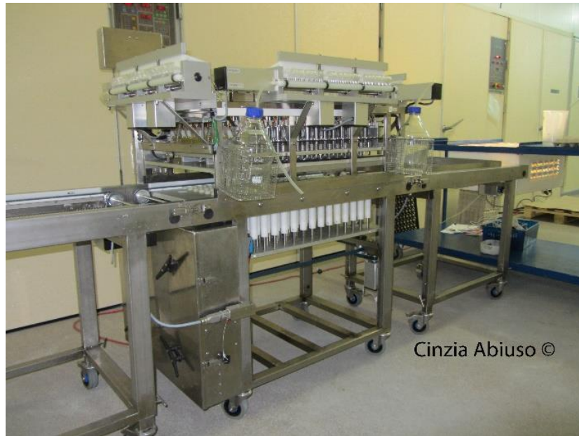
Figure 9.4 - In ovo injection with automatized system
