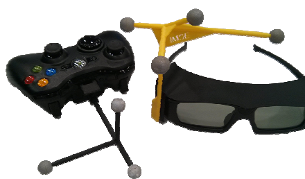
Figure 2, the primary user has a gamepad. Both the gamepad and the 3D glasses have a "target".
