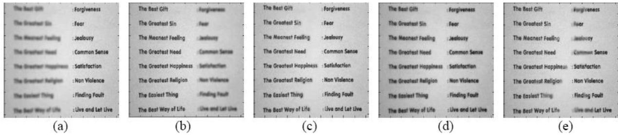
Fig. 6. Fusion results of multi-focus image of text (a), (b) Multi-focus source images (c) Proposed method (d) DWT method (e) Region method
