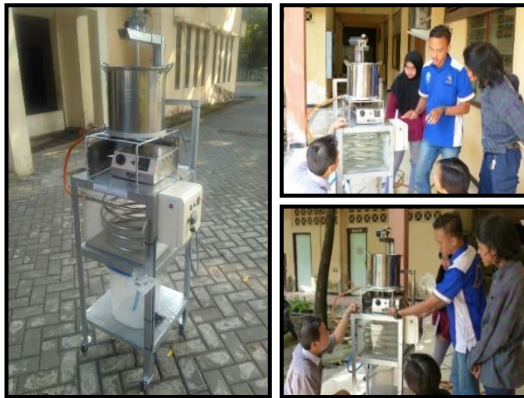
Figure 3. (MP3 SUPI) Processing Machine and Cow Milk Packer with 3 in 1 Integrated System
