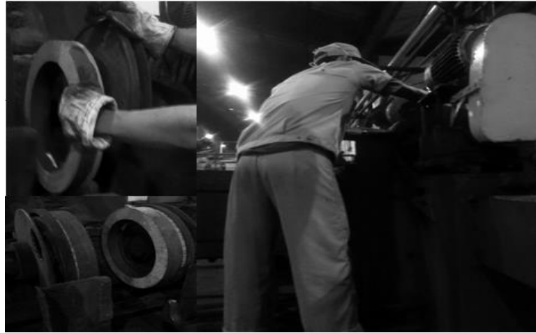
Gambar 1.2 Set up Pergantian Batu Gerinda
