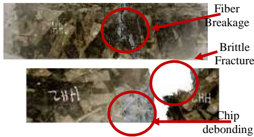
Fig. 4 Damage of DCFC (Feraboli et.al, 2009)
