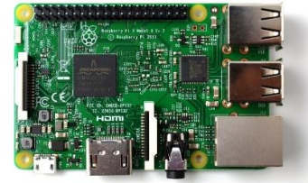
Gambar 7 board raspberry pi 3
