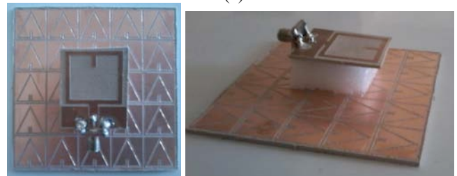
Fig. 9. a) Configuration of cpw antenna with an AMC reflector, b) Photograph of the fabricated AMC with antenna on top: left (top view) and right (side view).
