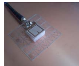
Fig.12. Measurement setup for the proposed antenna over large metallic surface
