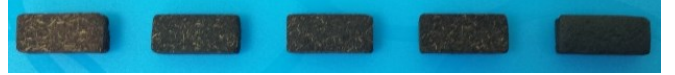
Figure 2: Fabricated samples of coir, 5wt% charcoal, 10wt% charcoal, 15wt% charcoal and charcoal respectively from left to right
