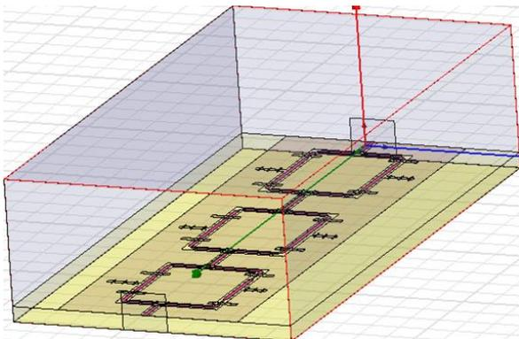
Figure 11: Schematic of the 3-bit integrated phase-shifter structure built in HFSS.
