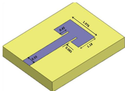
Figure 12: Geometry of the patch antenna
