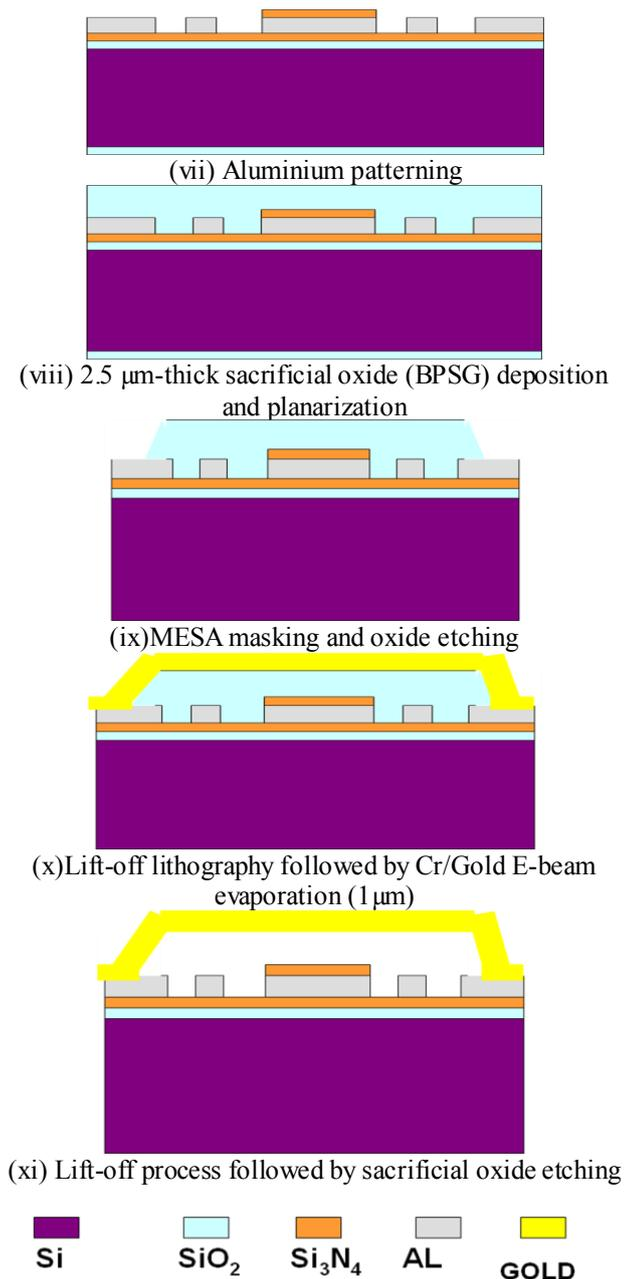
Figure 15: Proposed process flow for phased array fabrication
