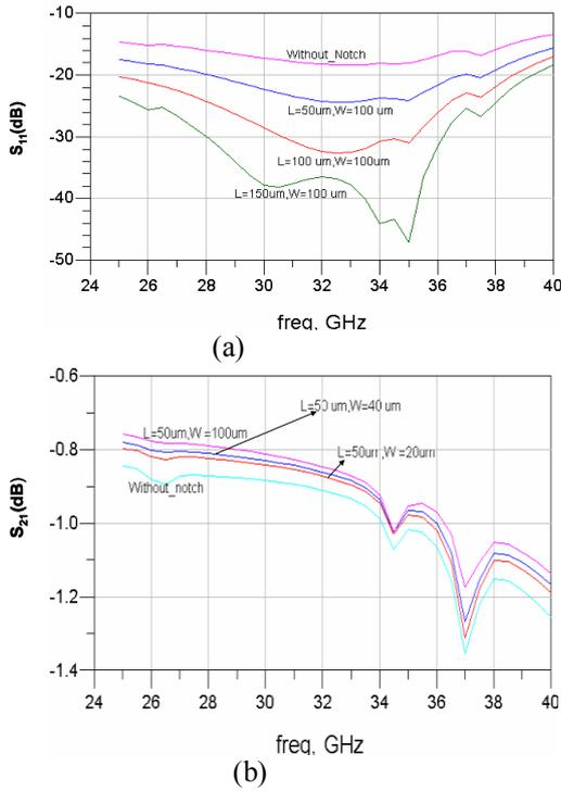
Figure 8: (a) Return loss performance with fixed width/variable length notches (b) Insertion loss variation with fixed width/variable length notches
