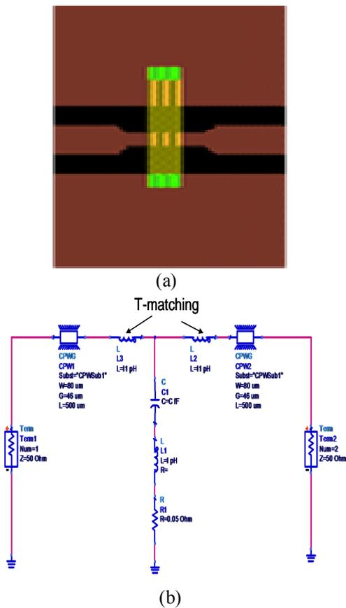
Figure 5: Layout for the T-match circuit (a) and equivalent circuit (b).
