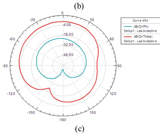
Figure 13 : Simulated (a) return loss (b) Peak directivity and (c) far-field radiation pattern of the patch antenna
