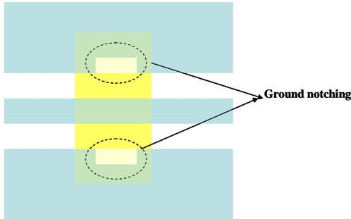
Figure 9: Layout of RF-switch with notched CPW ground
