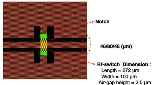
Figure 7: Notch introduced capacitive type shunt RF-switch structure
