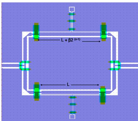
Figure 3:  $n^{\text{th}}$  bit layout of the phase shifter
