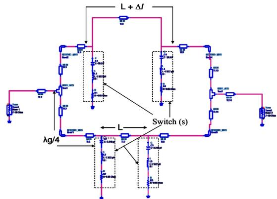
Figure 10: Equivalent ckt. of the single bit phase shifter
