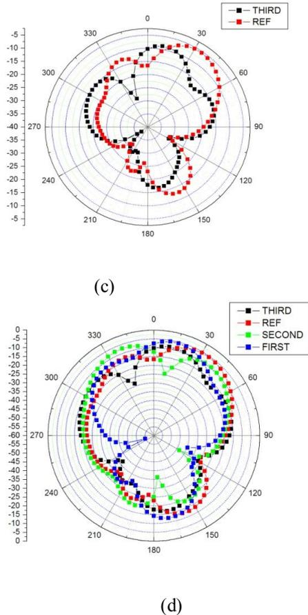
Figure 14: Scanning of the antenna beam with respect to (a) 1<sup>st</sup> bit (b) 2<sup>nd</sup> bit (c) 3<sup>rd</sup> bit (d) composite effect
