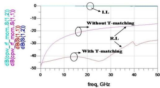
Figure 6: Improvement of RF performance by T-match circuit
