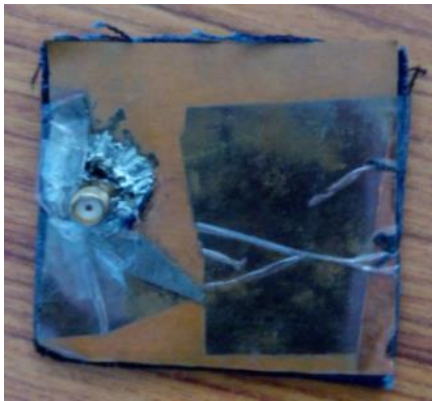
Fig.1.17 Rear view of fabricated antenna
