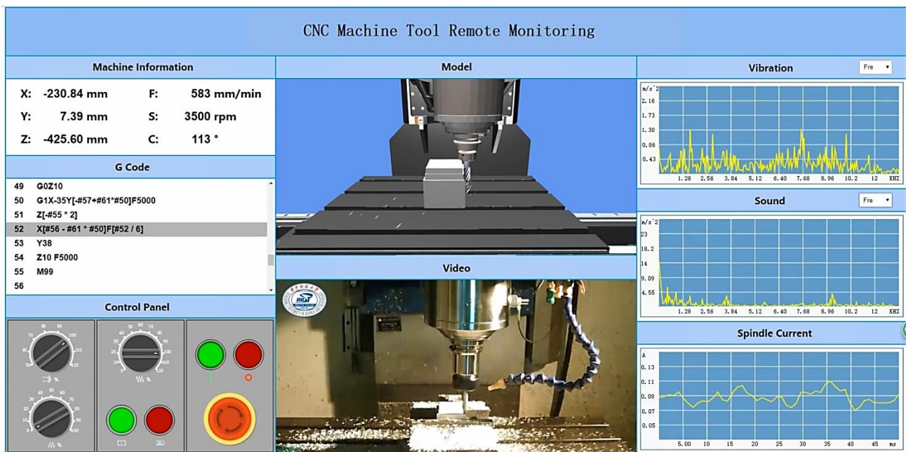
Fig. 6 Interface of remote monitoring prototype system based on HTML5
