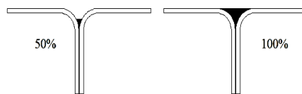
Fig. 6 Schematic of the adhesive fillet geometries for the T-peel joint [10]
