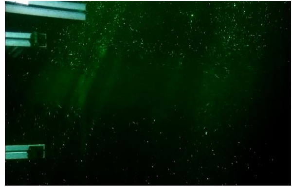
(b) PIV flow visualization
