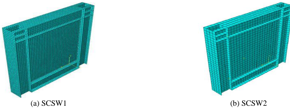
Fig. 5 Simulated models after meshing
