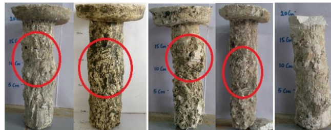
Fig. 8 Deformed shapes of stone columns (for Stone aggregate, Unreinforced stone column with Slag, Reinforced stone columns with spacing of 5.0cm for different embedment lengths of D, 2D and 3D/4D respectively)
