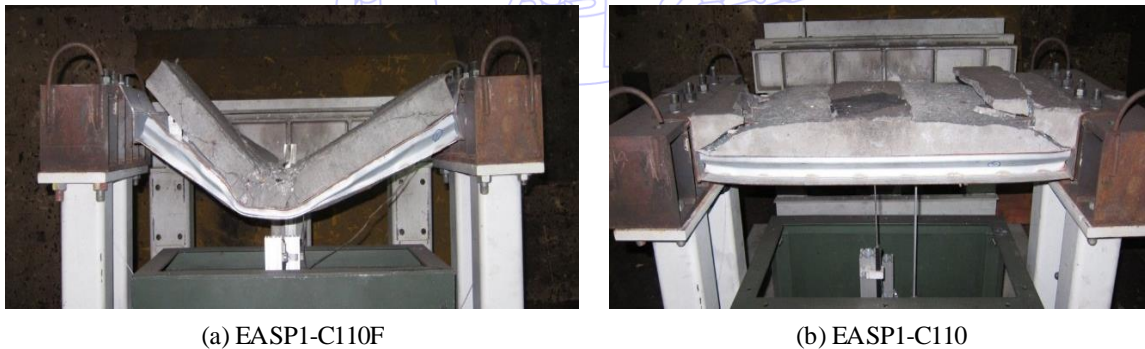
Fig. 8 Specimens after blast test
