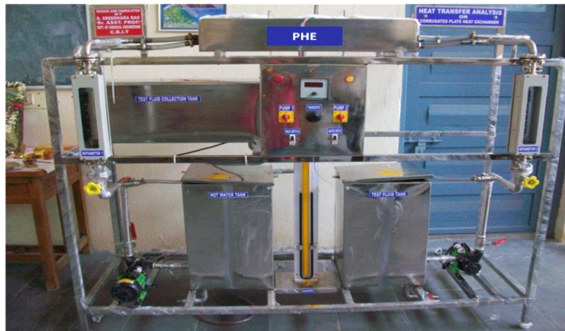
Fig. 1 Experimental setup of plate heat exchange
