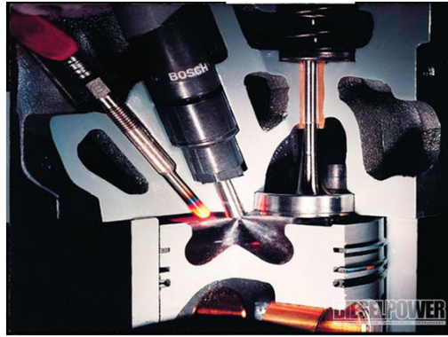
Fig. 1 Typical HDT Diesel direct injection combustion chamber [26]
