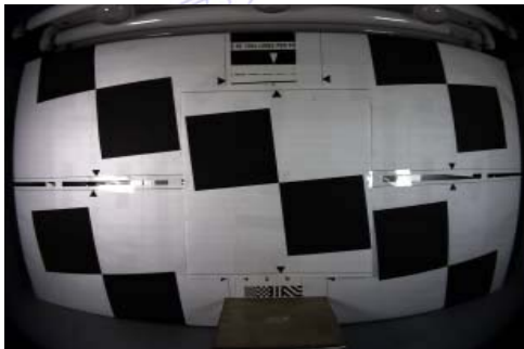
Fig. 17 Resolution Confirmation of Lens Shooting Chart
