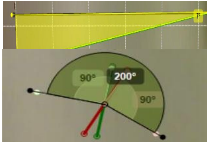
Figure 3. Technique used to measure angle changes. Green objects represent the initial heading and red objects represent heading after the angle change. Black angle measures the actual angle rotated.
