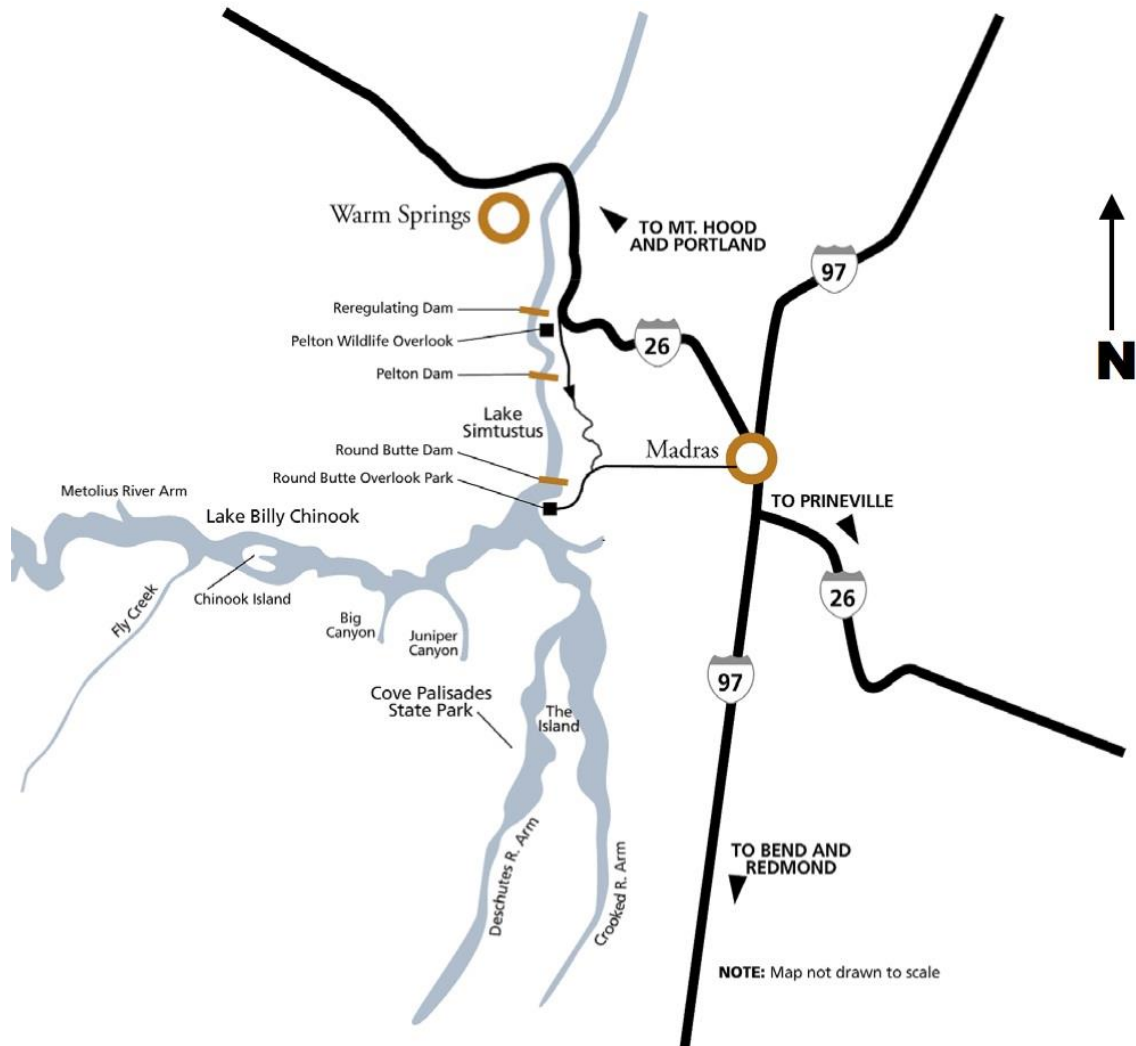
Map of the dams composing the Pelton Round Butte hydroelectric complex and resulting reservoirs. Swirling currents in Lake Billy Chinook resulting from temperature differentials between Deschutes and Crooked River water meeting colder Metolius River water hamper fish passage. 134
