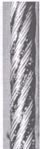
Fig.2b: Properly lubricated wire rope sample having fibre main core
