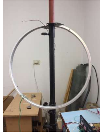
Fig. 4. One of the loop antennas constructed.
